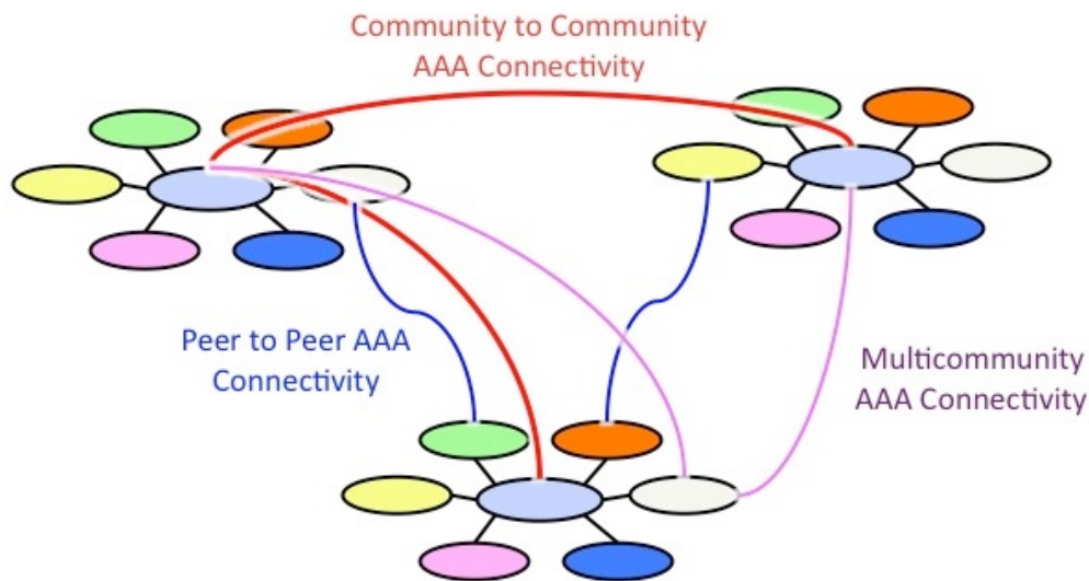
Figure 4: AAA Connectivity Architecture
